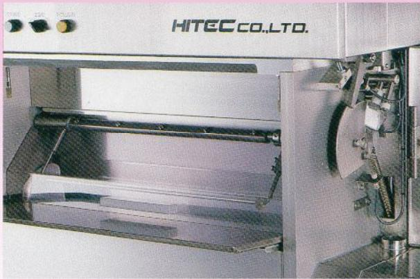
Charge the material meat into the opening in the picture above. The maximum length of material ham to be charged is 720 mm. Unless the safety cover is closed after material meat is charged, the upper mould press cylinder does not operate so that it is quite safe. Material meat held between the upper and lower moulds will be strongly pressed with the cylinder from above. So the material meat shall be shaped as per moulds and the well-shaped products will be manufactured.
