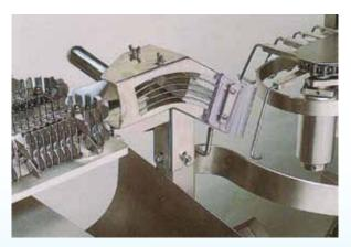
A revolutionary breakthrough over the conventional looper horn which moves to hang product over J-hooks.
