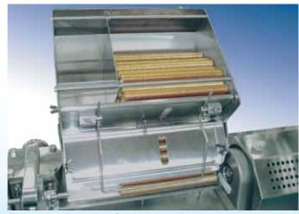
Flapper style casing feed mechanizm (Patented in the U.S.A.)
