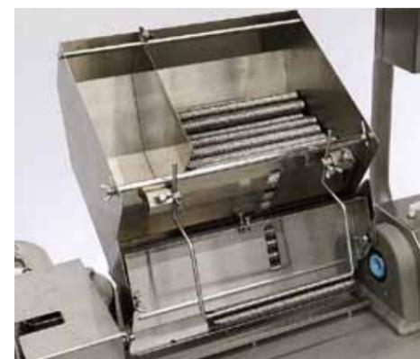
▶ **Flapper style casing feed mechanism**
