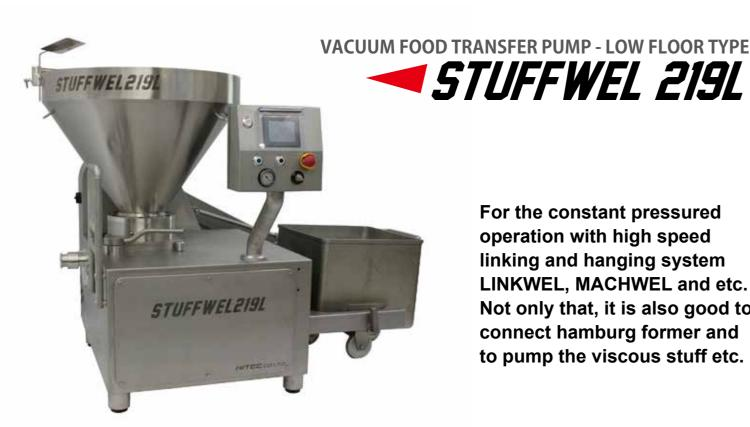
For the constant pressured operation with high speed linking and hanging system LINKWEL, MACHWEL and etc. Not only that, it is also good to connect hamburg former and to pump the viscous stuff etc.
