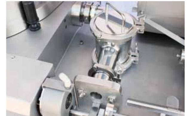
**Direct Piping (with Magnetic filter)**
